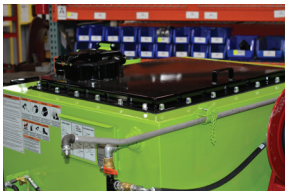
Tank Access Cover
