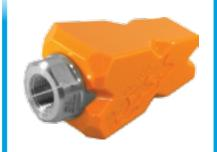
The new HXXpose<sup>™</sup> nozzle from Vactor blasts with a 0 degree stream of water up to 3000 PSI while rotating at a high speed to provide an 18 degree cone of coverage.
