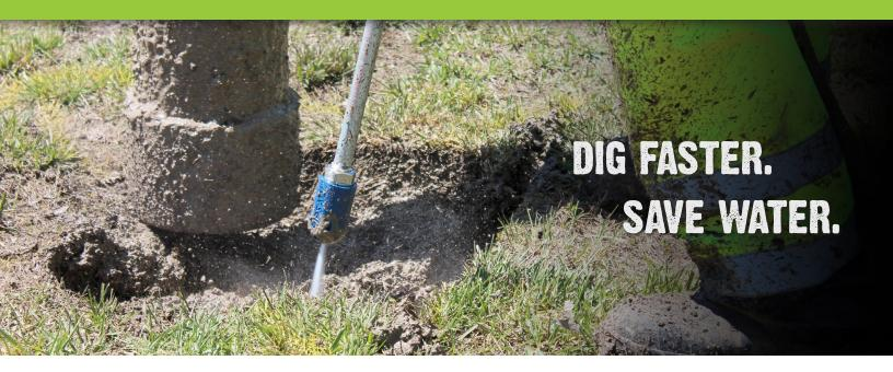
**PERFORMANCE** – The RIPSAW blasts a 0° straight water stream at up to 3200 PSI while rotating at an optimal speed to provide an 18° cone of coverage. The cone-shaped flow pattern is ideally suited for potholing applications.
